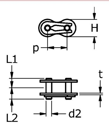
Breaking power = 4720C = 8.2d = 2.31D = -For chain size =  $8 \times 3$ For chain type = 05 B-1L1 = 3.8L2 = 4.7
